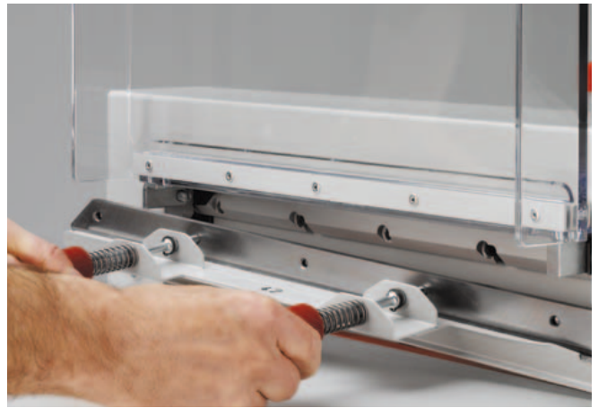
BLADE CHANGING DEVICE Safe and convenient blade change without removing machine covers: blade changing device with covered cutting edge.
