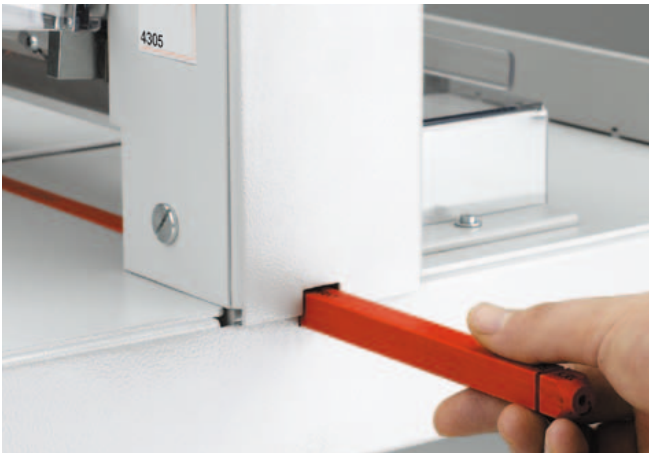
CUTTING STICK CHANGE On our office guillotines the cutting stick can be turned or replaced easily from the outside of the machine.
