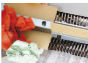
Crumpled paper is fed into the shredding unit by rotating rubber paddles in the feeding hopper of this shredder model.
