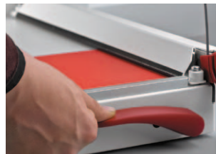
EASY_LIFT guarantees an easy and convenient removal of the paper from the cutting table by lifting the automatic clamp after the executed cut.
